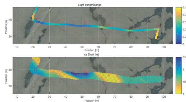
A coordinated survey with the new NUI H-ROV revealed different length scales of variability and enabled a statistic description of light transmission based on the physical properties.
