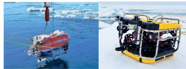
Operating ROVs under sea ice changes various paradigms of ROV operations as compared to bluewater operations. Heavy tether and vehicle trim as well as specialized navigation solutions are necessary for a smooth scientific investigation of the bottom side of sea-ice. In spite of the challenges, ROVs provide a great tool for interdisciplinary sea ice science.
