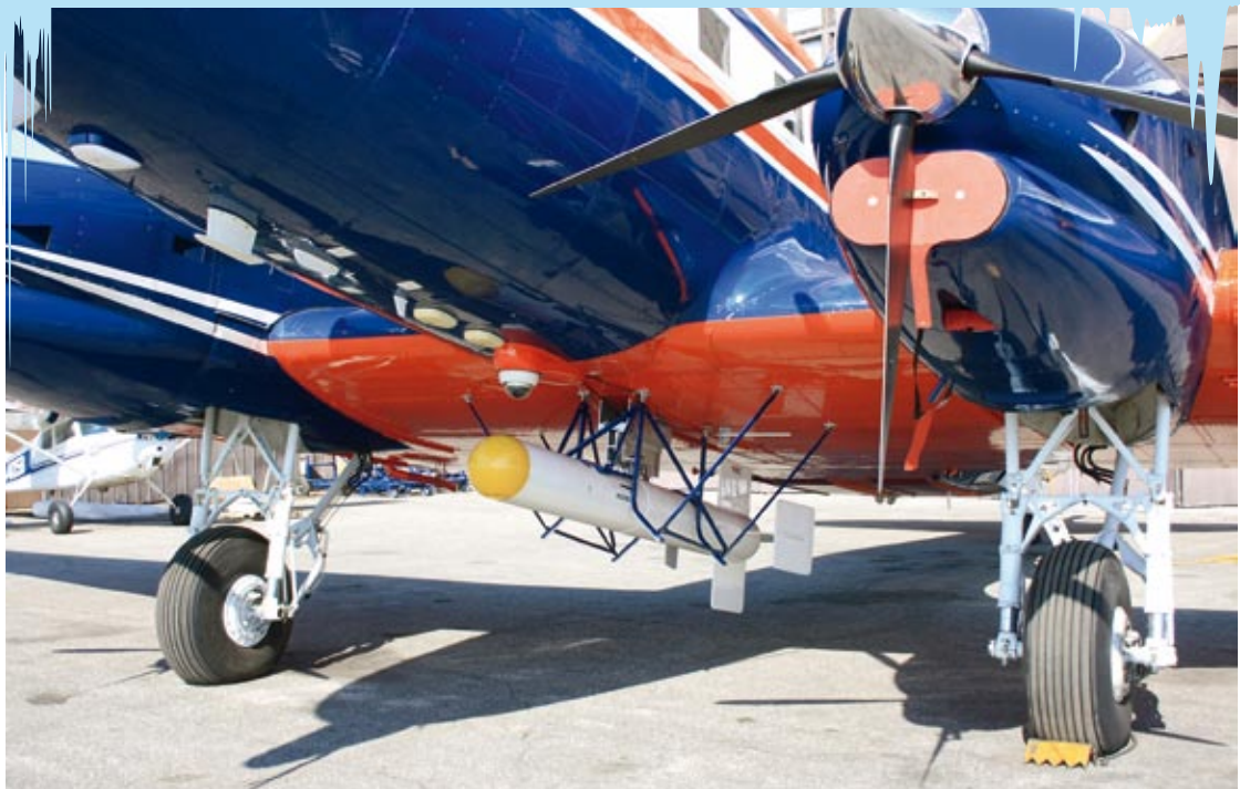
Fig 1: Towed sensor for determining the thickness of sea ice on the fuselage of the polar research aircraft 'Polar 5' in Fairbanks, Alaska Photo: Stefan Hendricks, AWI
