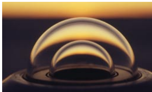
Fig 2: Glass domes of a pyranometer during the polar night at Neumayer. The pyranometer serves to measure solar and diffuse sky radiation. Photo: Gert König-Langlo, AWI
