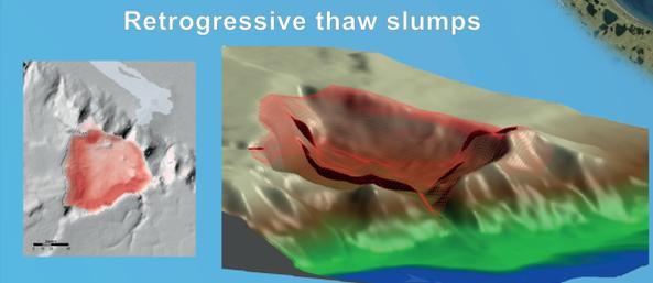
Active retrogressive thaw slumps released considerable amounts of sediments and caused coastline progradations up to 40 m.
