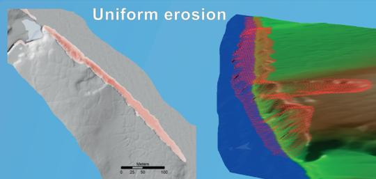
Uniform coastal erosion up to 20 m and little mass wasting in coasts lower than 10 m.
