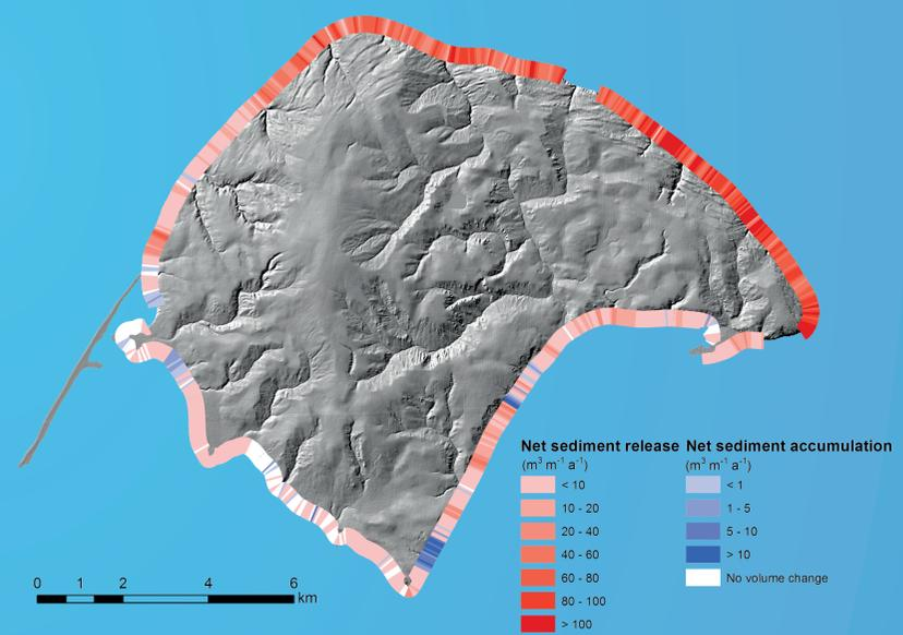
Volume changes derived from DEMs show less variability and more uniform patterns of coastal erosion. High volume decrease along north coast corresponds better with prevailing storm wind direction.
