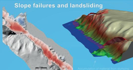
Mass wasting is very active on high coasts. Common are slope failures, slumping and active-layer detachments. Accumulation of material caused short-term coastline progradations up to 20 m.
