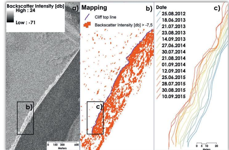
Monitoring cliff top retreat at the test site: a) TerraSAR-X scene from 21.08.2014 showing the test site; b) a threshold of -7.5 was defined by calculating the mean backscatter intensity within a ROI on the cliff. The threshold was applied to the TSX images prior to mapping of the cliff top; c) cliff top lines from TerraSAR-X images within the thawing season. Lines will be analyzed using the Digital Shoreline Analysis System developed from the USGS<sup>2</sup>.
