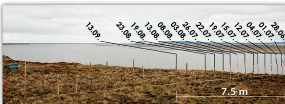
Time-lapse camera setup at the test site. We installed 29 wooden markers every 50 cm perpendicular to the cliff top and a Brinno TLC200 Pro time lapse camera viewing from South to North. Pictures were taken every four hours from 28.06.2015 to 13.09.2015. In that period 15 markers were eroded, equaling 7.5-m of cliff top retreat.
