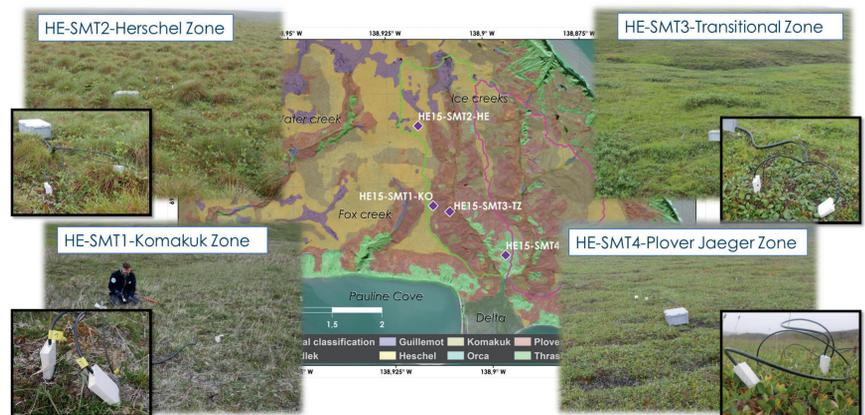
Four stations measuring soil moisture and temperature close to the surface were installed in July 2015 in four different landscape units to compare the influence of snow on the soil moisture dynamic. Each station has two soil moisture and temperature sensors each that are installed vertically and diagonal. Animal attacks of the stations are a risk.
