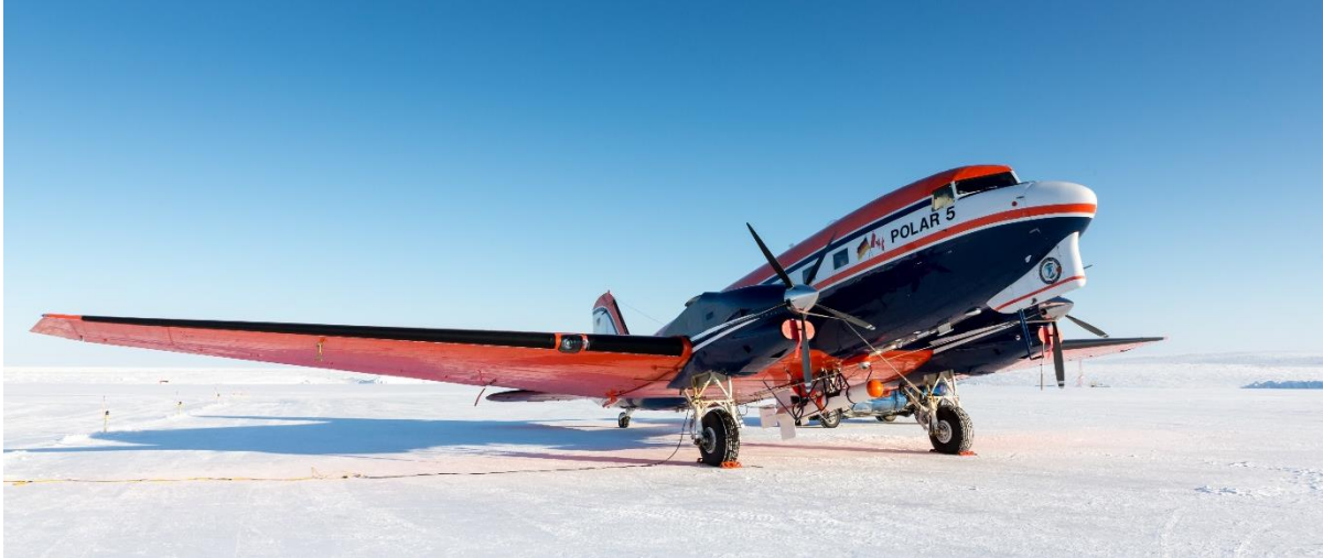
Figure 2: Polar-5, a polar research aircraft of the Alfred Wegener Institute outfitted with an AEM sensor for direct sea-ice thickness observations. York University operates are similar aircraft of the same model and scientific payload.
