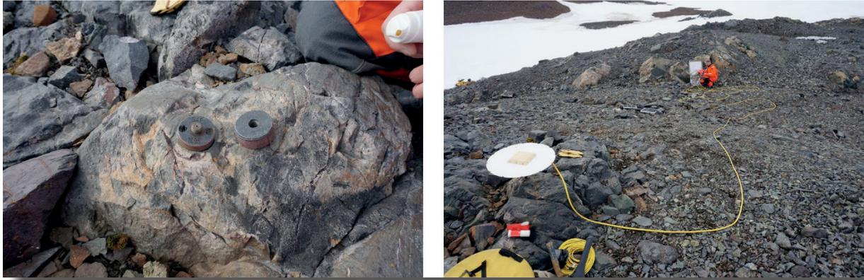
*Fig. 4.4.3: Installation of the GPS equipment at the sites PRA1. The left photograph shows the existing GAP (Geodetic Antarctic Project) marker from 1995. The right photo shows the mounted GPS antenna in the left foreground.*
