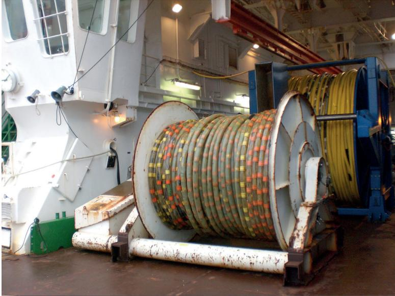
*Fig. 6.3.3: The 600 m long analogue streamer (front) (Type PRAKLA) (Photo: Sascha Plewe (IOW))*
