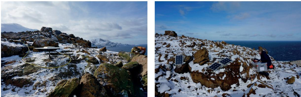
*Fig. 4.4.4: Installation of the GPS equipment at the sites ELE1. The left photograph shows mounted GPS antenna on the existing GAP marker from 1995. The right photograph shows the solar-panels (left) for power supply of the receiver and the Zarges aluminium box (right) to protect the receiver and battery.*
