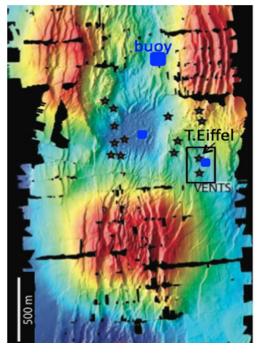
(Right): detailed bathymetric map of the volcano summit with the different hydrothermal vent sites (stars), the location of the Tour Eiffel edifice, of the 2 SeaMon nodes and of the relay buoy (blue squares). Seafloor depth are between -1550m (red) and -1770m (dark blue).
