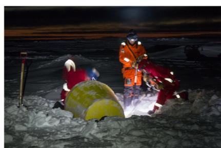
We dug ITP93 out of the snow and drilled/ picked it out of the fresh-water ice. Recovery by hand was impossible due to 2m thick ice and unclear tether position.
