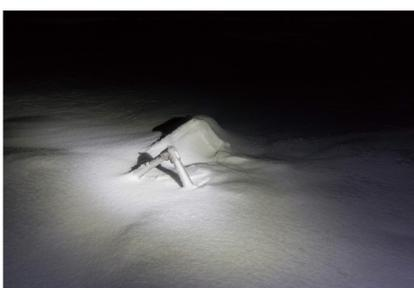
Only the datalogger unit of the spectral radiation station could be recovered. The station failed early during the measurement period and likely sunk into a meltpond.
