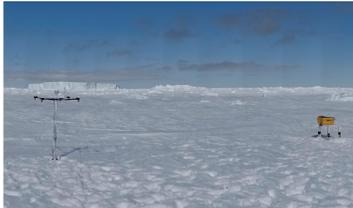
Fig. 3: Snow Buoy (left) and IMB (right), deployed on a sea ice floe in the Weddell Sea.
