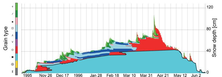
Fig. 5a: SNOWPACK simulations with sea ice domain using Weissfluhjoch meteorological forcing data. Sea ice is represented in cyan, the other colors indicate snowpack microstructure.
