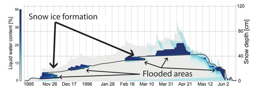
Fig. 5b: Liquid water content (LWC) of the snowpack, the model is able to represent flooding processes with LWC increasing up to 50% after new snow falls.
