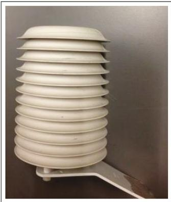
**Figure 2:** Combined air temperature and humidity sensor
