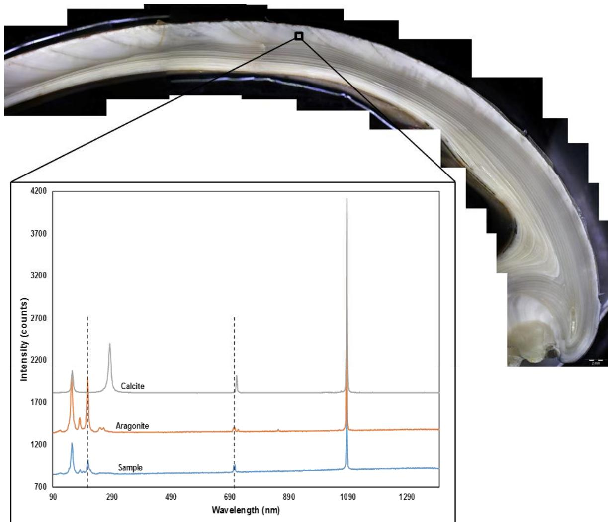
Figure 9: Confocal Raman microscopy (CRM): The black square indicates where one single spot measurement (three per ontogenetic years resulting in nine spectra per shell) was performed (specimen-ID VL-Siz-58). Scale-bar on shell cross-section is 2 mm. CRM clearly shows that the sample does not show signs of diagenesis. Sample (blue) and aragonite (orange) standard spectra show identical peaks whereas the calcite (grey) standard spectrum differs from the sample spectra.
