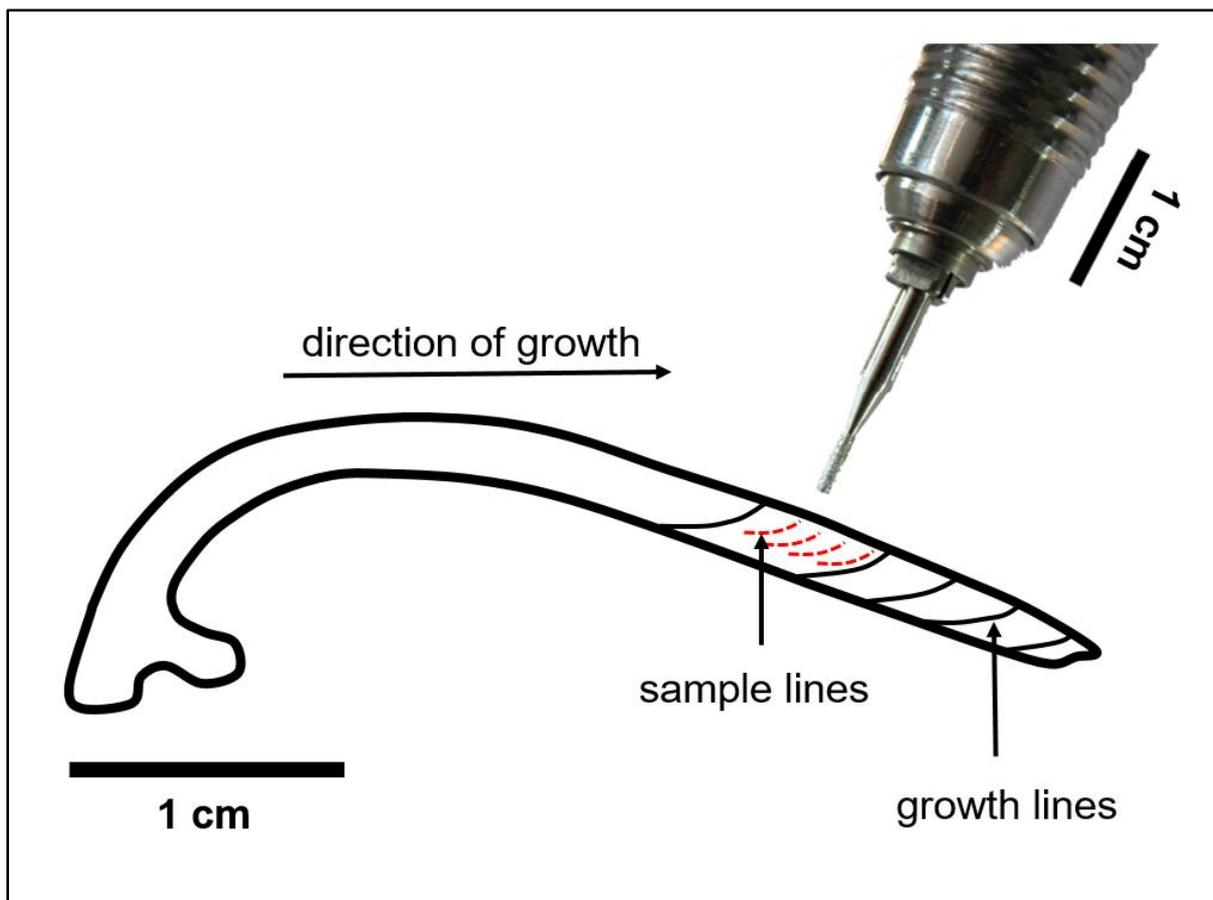
Figure 5: Micro-milling for  $\delta^{18}\text{O}_{\text{shell}}$  analysis. Calcium carbonate ( $\text{CaCO}_3$ ) samples were milled from the outer shell layer in three consecutive years using a 700  $\mu\text{m}$  mill bit.
