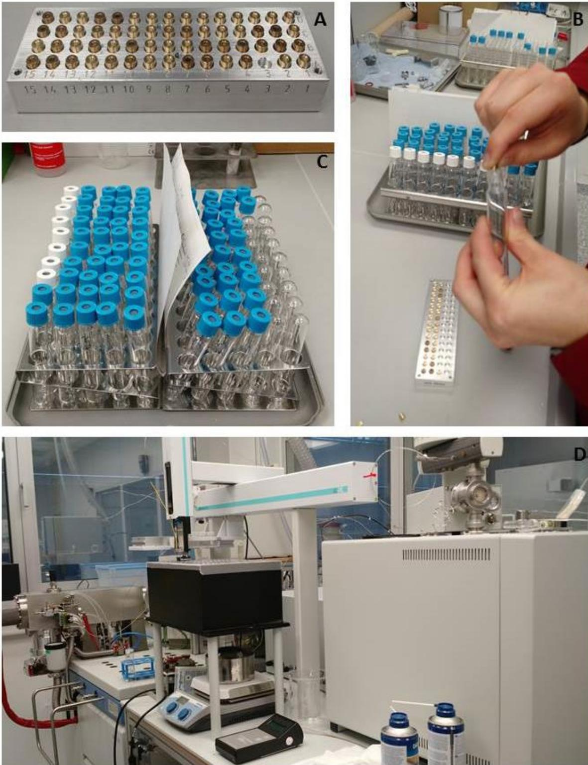
Figure 6: Isotope ratio mass spectrometry (IRMS). (A) Aluminium tray with crucibles and samples. (B) Transferring calcium carbonate sample from crucible to borosilicate exetainers. (C) Exetainers closed with special caps, which enable measurement without reopening. (D) Thermo Finnigan MAT 253 continuous-flow isotope ratio mass spectrometer equipped with a GasBench II at the Institute of Geosciences, University of Mainz, Germany.
