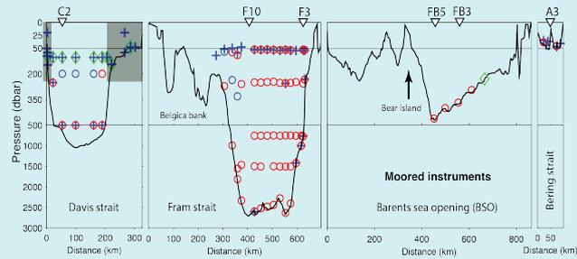
Fig. 1. Moored instrument locations during 2005-2006: Microcats (blue), RCMs (red), ADCPs (green). B11-B14 & WG1-WG4 in Davis Strait have not been analysed yet, and shaded in grey.
