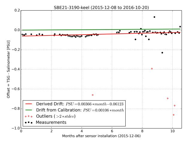
Figure 3: Sensordrift of TS Keel
