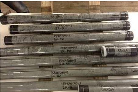
Fig. 2: MeBo drill cores with various layers of consolidated sediments. The cores are inside their plastic liners and will be split later for taking samples (Photo: K. Gohl)
