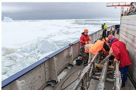
Fig. 2: The geology team pulls the inner core pipe of the gravity corer filled with sediments (Photo: T. Ronge)
