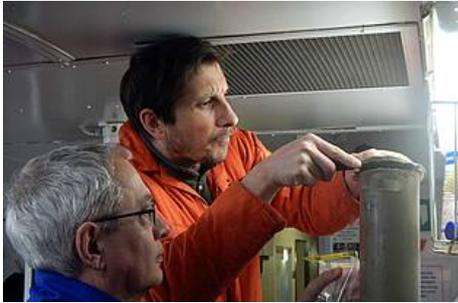
Fig. 3: James and Werner cut slices of marine sediments from the pipe of the multi-corer for further analysis (Photo: Alfred-Wegener-Institut)
