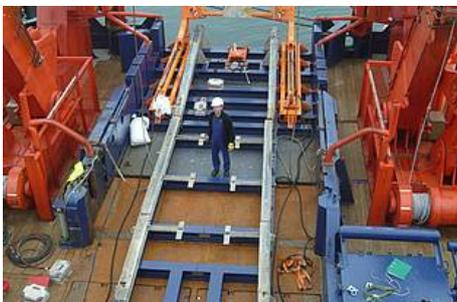
Fig. 1: Installation of the MeBo's launch and recovery system on the deck of POLARSTERN (Photo: Robert Larter)
