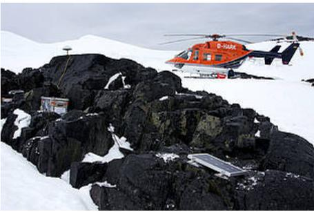
Fig. 2: A geodetic measurement station installed on Clark Island by Mirko Scheinert and Benjamin Ebermann (Photo: Mirko Scheinert)
