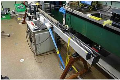
Fig. 3: Before the MeBo cores will be split they are scanned by the multi-sensor core logger to measure their physical properties (Photo: T. Frederichs)
