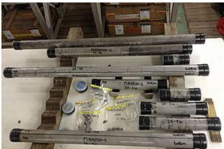
Fig. 1: Sediment cores from MeBo drilling from down to 30 m drill depth. After the physical properties of the cores are logged in a core logging unit, the cores will be split in two halves (Photo: Karsten Gohl)
