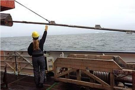
Fig. 6: Ricarda's temperature probe is returned to deck after its temperature sensors measured temperatures at various depths in the sediment to derive geothermal heat flux (Photo: K. Gohl)
