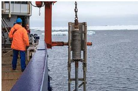
Fig. 1: The gravity corer is lowered into water to collect sediments from several metres deep in the seafloor (Photo: T. Ronge)
