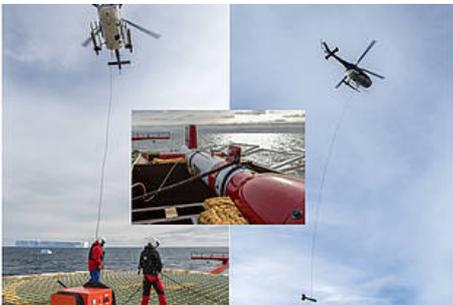
Fig. 1: The helicopter-magnetometer sensor on its mission to survey the Earth's magnetic field (Photo: T. Ronge)
