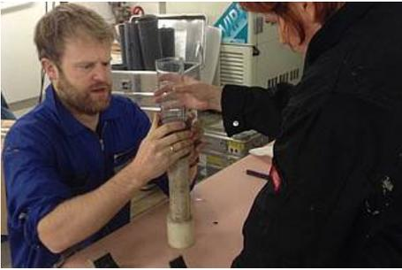
Fig. 5: Johann and Tina trying to push a tight-sitting sediment core out of its plastic liner (Photo: Karsten Gohl)
