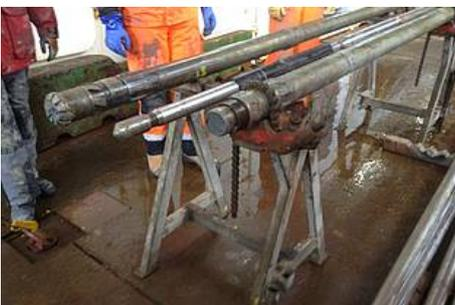
Fig. 4: MeBo drill string with a drill bit to the left of the photo (Photo: Karsten Gohl)
