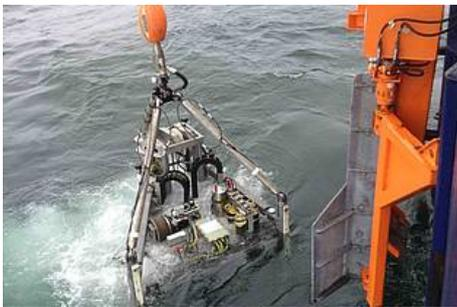
Fig. 1: The MeBo on its way to 1000 m depth (Photo: Karsten Gohl)
