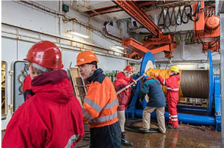
Fig. 4: The 600 m long seismic streamer is deployed (Photo: T. Ronge)
