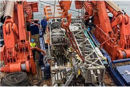
Fig. 2: The MeBo is lifted onto its launch and recovery system (Photo: Thomas Ronge)
