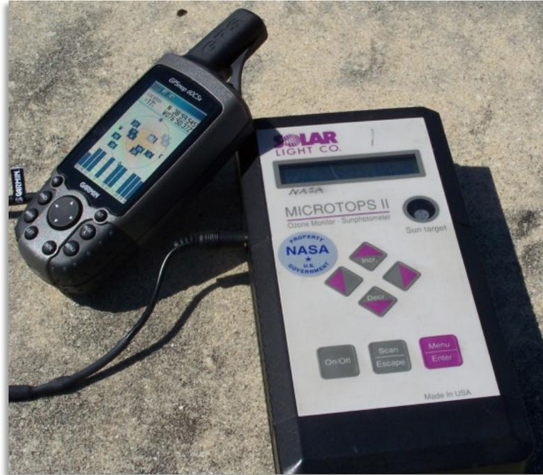
Fig. 3.1: Calibrated Microtops and GPS unit provided by NASA's Marine Aerosol Network
