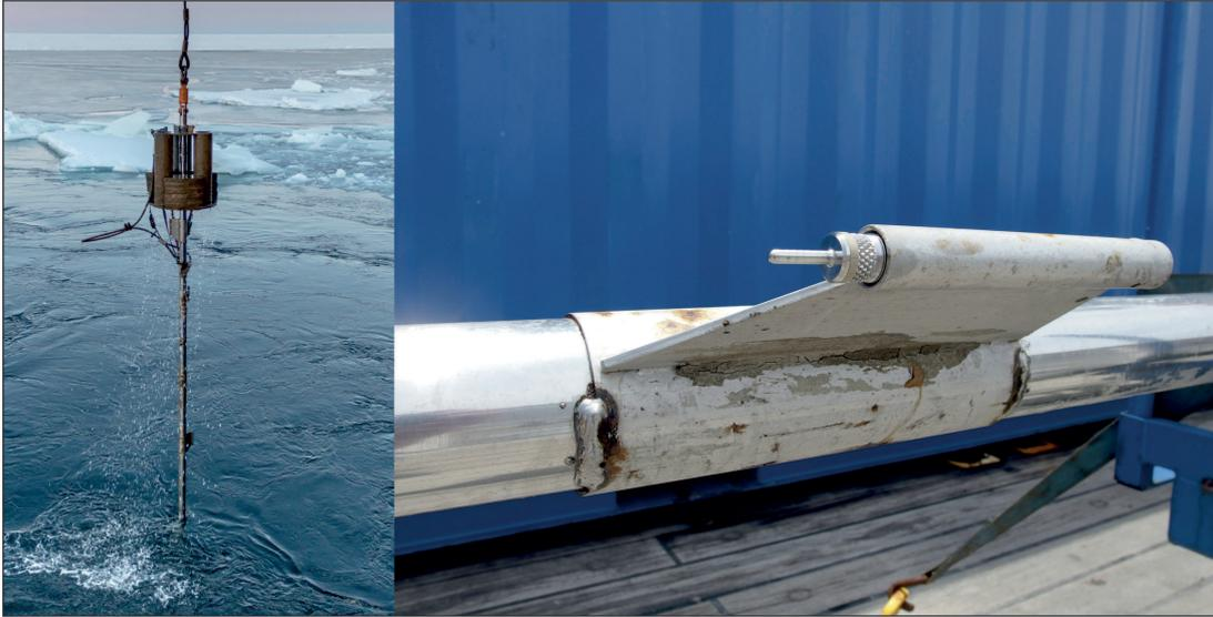
*Fig. 5.1: The 5 m long temperature lance immediately after recovery with six miniaturized temperature data loggers mounted on the outside wall of the strength member (left). MTL in clamp mounted on the temperature lance (right).*
