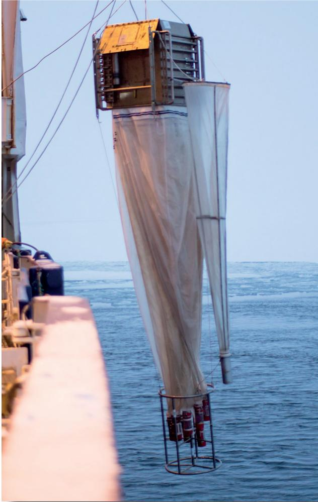
Fig. 7.1: The Multinet Maxi with the attached side net.
