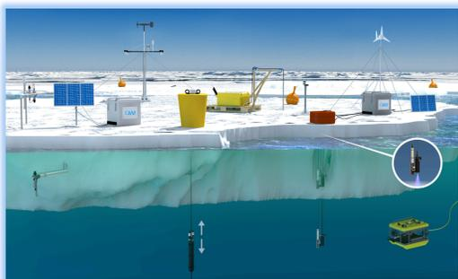
**Ice buoys and ice-tethered platforms** installed on ice floes in the central Arctic Ocean measure solar radiation, albedo, snow height, ice thickness, temperature, and algal activity. The data are delivered year round in partly near real time. The AWI sea ice buoy network is part of an international effort. An newly developed **under ice ROV** with extensive sensing capabilities provides unique pictures of the under ice world and can be used for many manipulation / intervention tasks.
