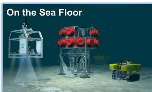
The **modular benthic observatory** consists of a **towed camera system (OFOS)**, a **benthic lander** system and an **autonomous crawler (TRAMPER)**. Visual observations, biogeochemical flux studies and ecological experiments give long term information on so far unknown processes at the deep seabed. The towed camera system is part of the Pollution Observatory, photographs of the sea floor have shown a strong increase of plastic litter on the Arctic Sea floor.
