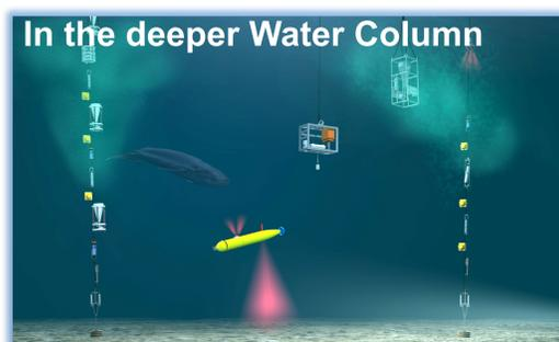
**Multidisciplinary techniques** are combined to study particle biogeochemistry, zooplankton ecology, marine mammals, and the physical and environmental characteristics: Moored **BioOptical Platforms** are completed by ship based particle cameras and traditional traps. The **high resolution zooplankton camera LOKI** is operated from ship to investigate spatial distribution. Highly **precise hydro-acoustic recorders** locate marine mammal sound.
