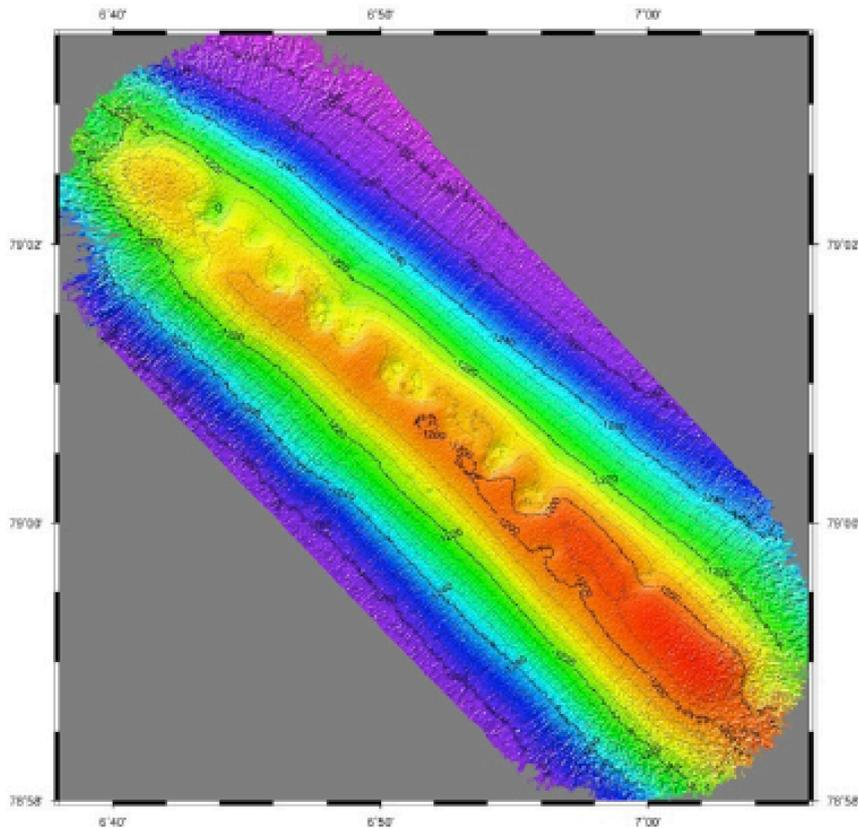
Fig. 4.2: Multibeam image of the working area. Pockmark depressions are clearly visible
