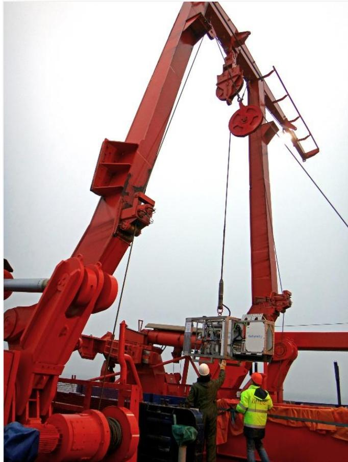
Figure 2-9: OFOBS subsea unit launched with the A-frame of *RV Polarstern*. Deployment is possible over either the side or the stern of the ship. (Photo: Laura Hehemann)
