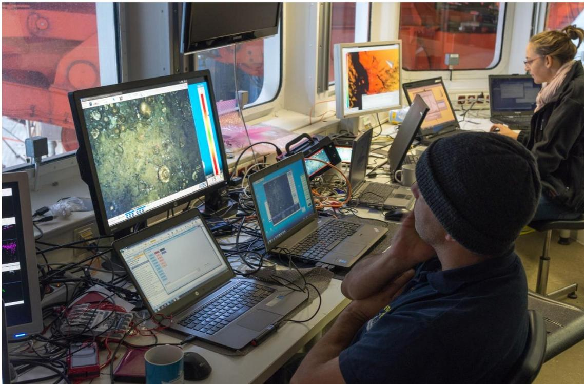
Figure 2-10: The OFOBS workspace during a dive on PS101. (foreground) The scientific observer keeps an observation log and controls the manually triggered still image recordings. (background) The GIS operator monitors ship and vehicle tracks for station planning purposes.
