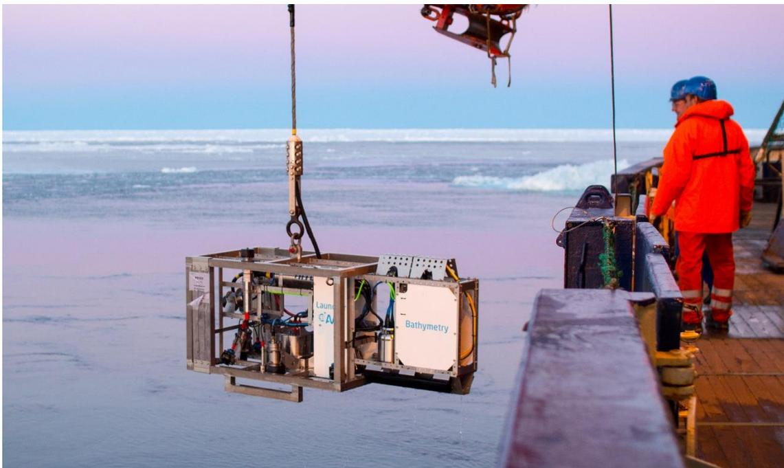
Figure 2-1: OFOBS subsea unit coming back on deck of *RV Polarstern* (Photo: Frederic Tardeck)
