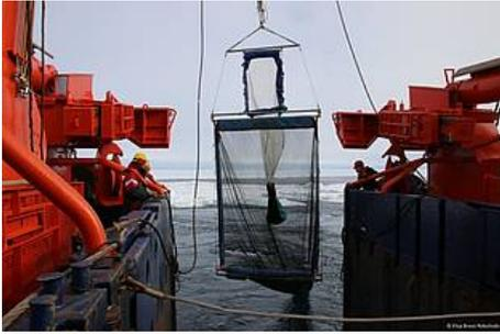
Fig. 3: Mounting the Surface and Under-Ice Trawl (SUIT) before its first deployment. (Photo: Elisa Bravo-Rebolledo)
