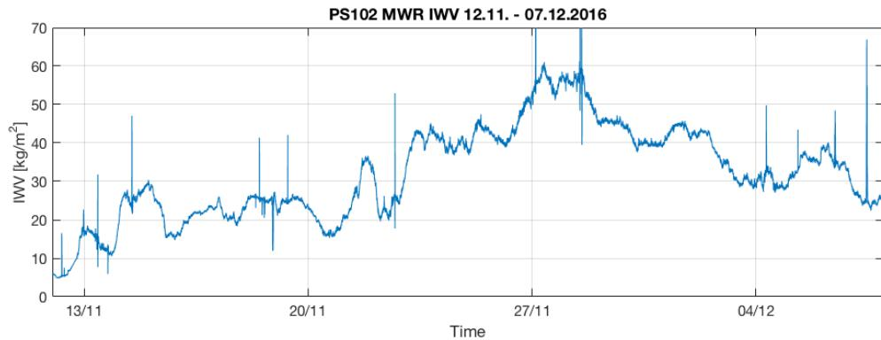
*Fig. 5.3: Integrated water vapour (I WV) during PS102 measured with the microwave radiometer HATPRO*
