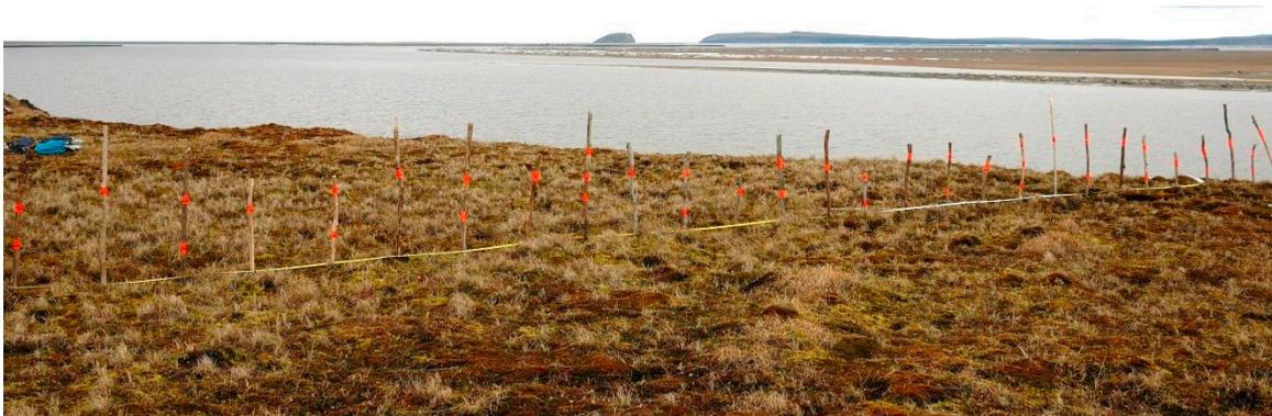
**Figure 5.** Monitoring of cliff-top erosion on Kurungnakh Island. The field photo from 21 June 2015 shows the field of view of the time lapse camera on the eroding cliff top. The camera monitored a 15 m long transect that was set up perpendicular to the cliff-top line and consisted of 29 equally spaced (50 cm apart) wooden stakes. Photo: Samuel Stettner, June 2015.
