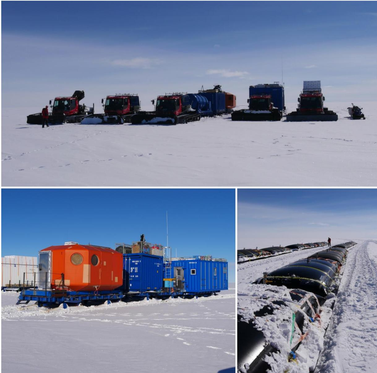
*Fig. 5: Top: The traverse car park. Five PistenBully® track vehicles and a Ski-doo® motor sledge parked closely next to each other in a lunch break. Every 50 km the vehicles had to be refueled. Bottom left: Living container for maximum six persons. Inside there is a small entrance area, in the back is a table with three bunk beds. Bottom right: bladder tanks on sledges with 80,000 liters of fuel.*
