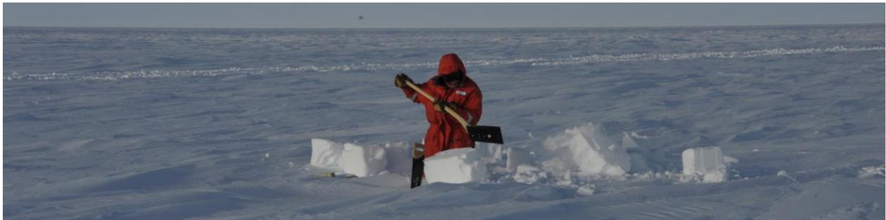
Fig. 7: Digging a snow pit at location 16. In front of the snow pit the liner is already inside the snow, its top is covered with a wooden plate. To dig a snow pit efficiently, it is advisable to saw blocks with a hand saw and lift the blocks with a shovel out of the pit (credit: Sepp Kipfstuhl).
