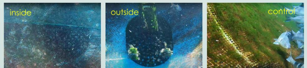
View of the inducers from the inside and outside of the ultrasound treated nets compared to control (pictures by Murat Arkut)
