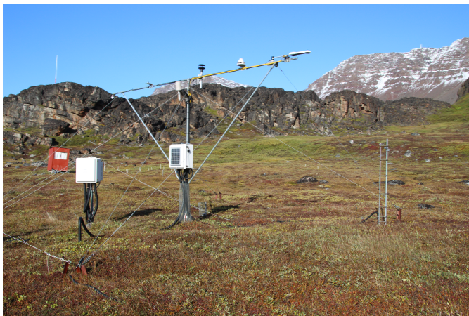
(a) AWS2 near the Arctic Station. The pyranometer in (b) is mounted on the right end of the horizontal pole, 15 th September 2023.
