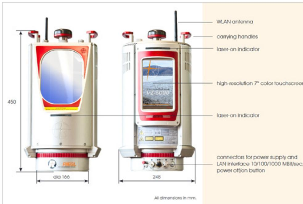
Fig. 4.22.1: RIEGL VZ<sup>®</sup> - 6000: operating elements and connectors (RIEGL, 2020)
