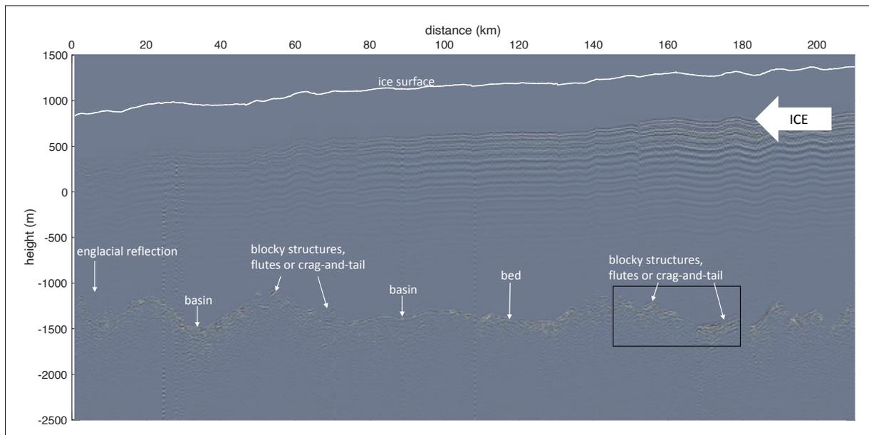
*Fig. 5.2.3: Throughout the 208 km profile we see blocky structures identified elsewhere as flutes or ‘crag-and-tail’ features. We see englacial reflections some 200 m above the bed on the far-left side, fading out and reappearing at km 160–180. We see several basins, a large one, 20 km long, 110 m deep, at km 90. The inset box, also showing these blocky structures, has been surveyed before by Muto et al. (2019).*
