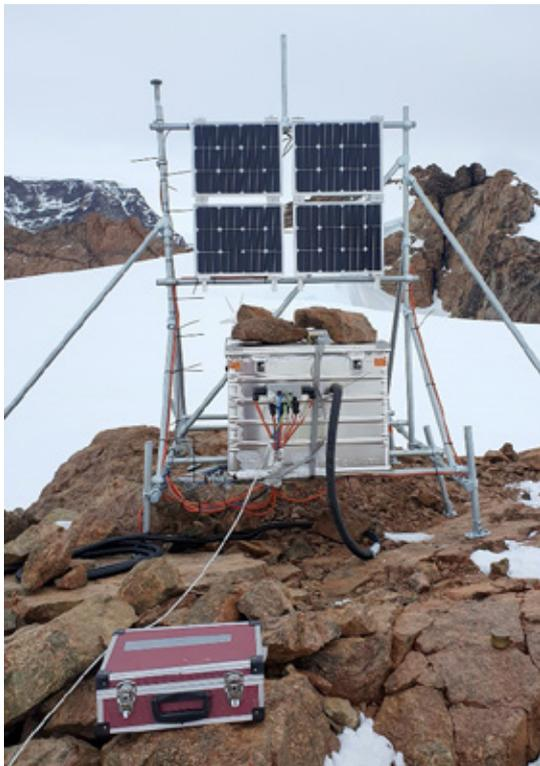
Fig. 4.25.3: Setup of the permanent GNSS station KOP1 at Weigel Nunatak (Kottas Mountains).
