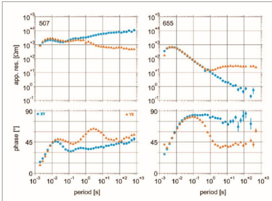
Fig. 4.14.4: Preliminary results (sounding curves) of the magnetotelluric measurements; the diagram on the left shows apparent resistivity in [ $\Omega\text{m}$ ] and phase curves in [ $^{\circ}$ ] over period in [s] of site 655, the data on the right-hand side are from site 507. The different colours indicate the two main directional components, which would lie on top of each other in case of a one dimensional subsurface.
