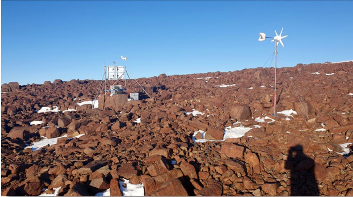
Fig. 4.25.2: Setup of the permanent GNSS station FOP1 at Forstefjell.
