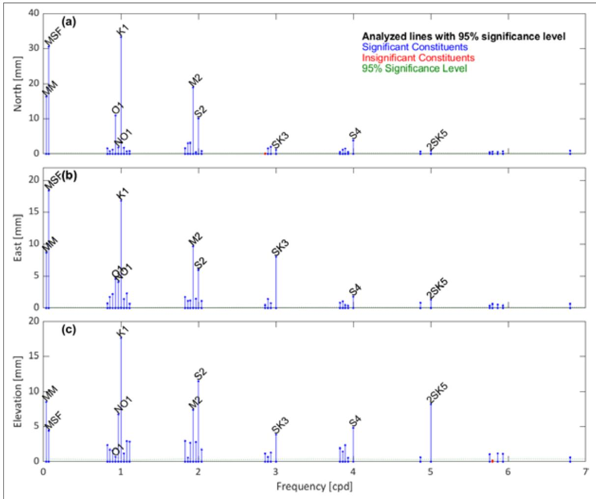
Fig. 4.14.3: Amplitudes of the tidal ice movement at GPS02 for (a) the north, (b) the east and (c) the high component
