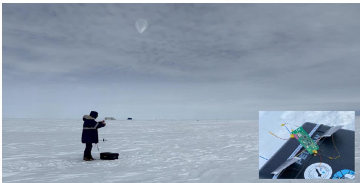
*Fig. 4.21.1: MSPB shortly before launch. Right figure shows one of the WSPR balloon trackers.*
