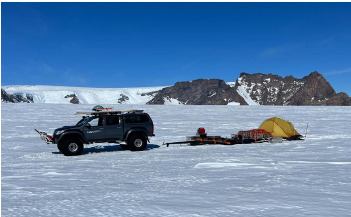
*Fig. 4.25.5: Usage of Toyota Hilux Arctic Truck together with PE mat. At the PE mat, the tent was temporarily set up for overnight accommodation.*
