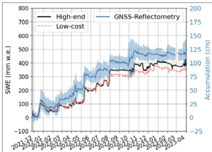
Fig. 4.13.1: Derived timeseries from GNSS reflectometry and refractometry for accumulation and SWE
