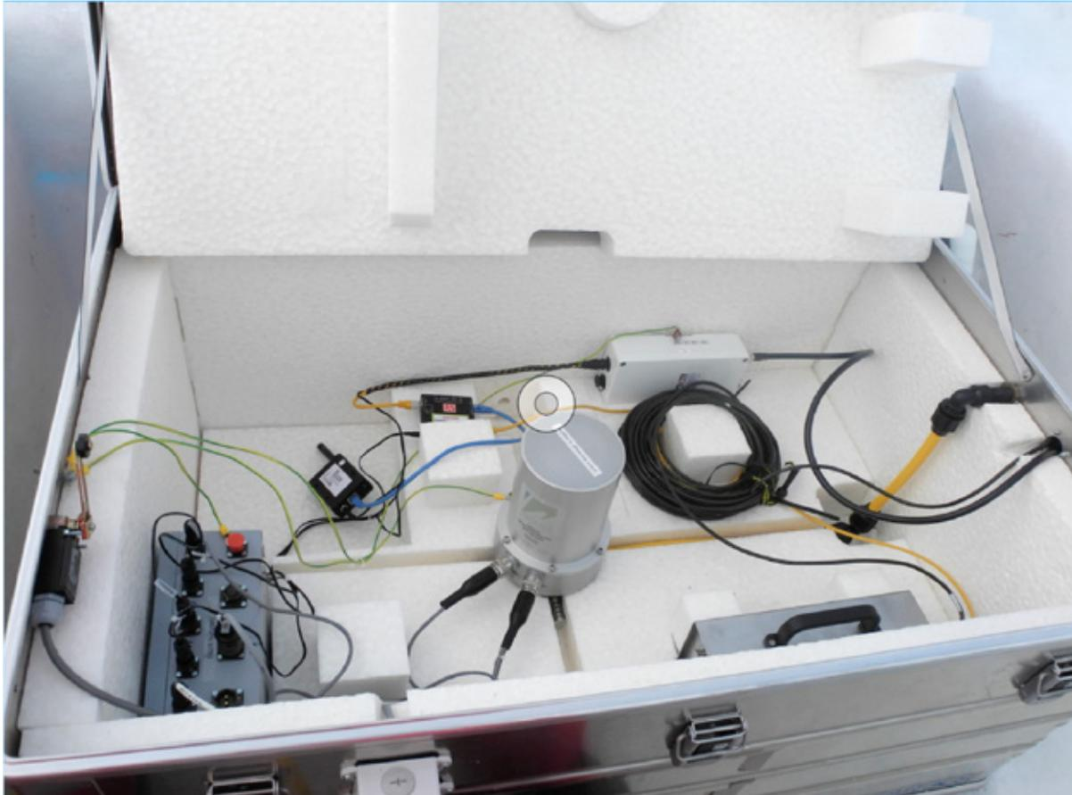
*Fig. 4.4.3: The insulated field-box contains the microbarometer (in the middle), data acquisition system as well as the power supply and a communication unit.*
