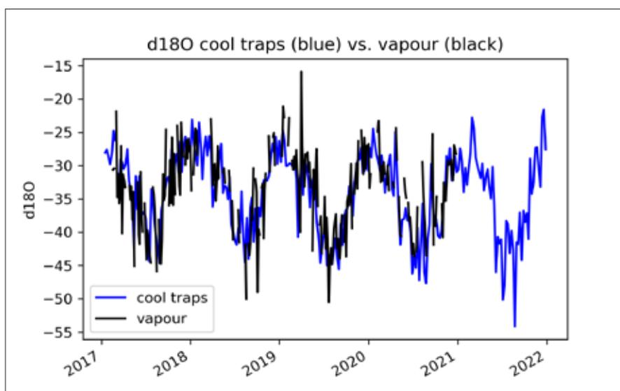
Fig. 4.29.2: Isotope  $\delta^{18}\text{O}$  variations measured at water samples collected from cold traps (blue line) and measured directly in vapour (black line) at Neumayer III Station during the years 2017-2022 (unpublished figure by M. Hoerhold and M. Behrends, AWI, 2023).
