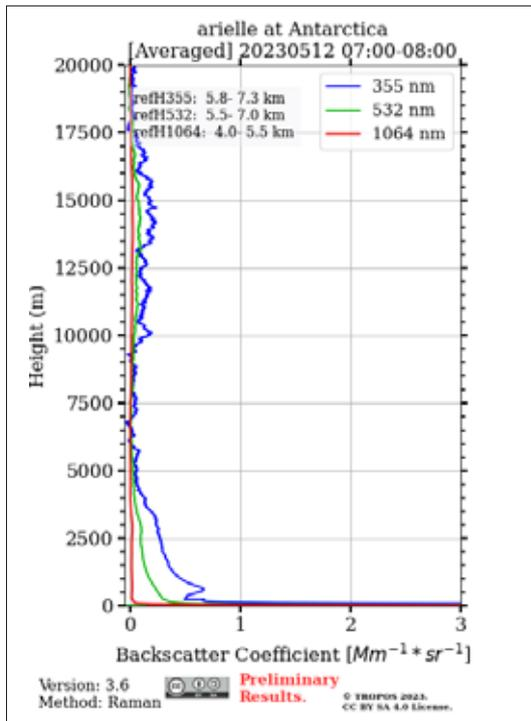
Fig. 4.20.3: A quicklook of the three-wavelength backscatter coefficient profile from aerosol measured above Neumayer Station III with the Raman lidar on 12 May 2023 between 07:00 and 08:00 UTC (<https://polly.tropos.de>). Two distinct aerosol layers are visible; free-tropospheric aerosol at altitudes up to 6 km and a high-altitude plume from 9 – 18 km height, presumably remnants of the 2022 Hunga Tonga–Hunga Ha’apai eruption in the Tongan archipelago.
