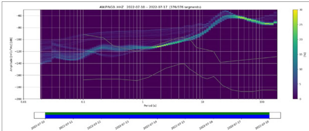
Fig. 4.17.2: Periodogram of two components of the seismometer.
