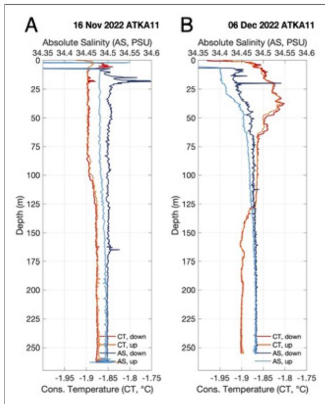
Fig. 4.6.6: Profiles of absolute salinity and conservative temperature for the down- and upcast respectively (dark/light blue, red/orange) at ATKA11 on (A) 16 November and (B) 6 December 2022.
