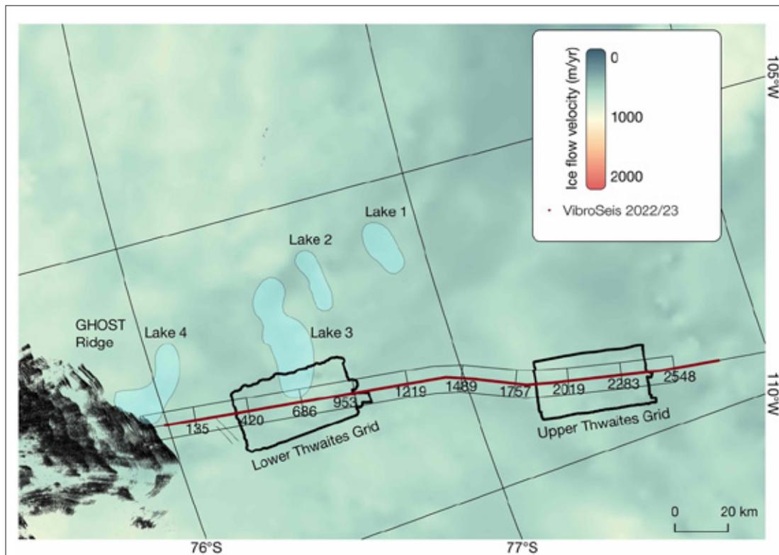
*Fig. 5.2.1: The survey boxes of Thwaites Glacier and the recorded seismic centerline profile (red). The area of the black curved shadowy lines on the bottom right side is the crevasse zone, partly covering box 1. Two big crevasses cross the lower (west) side of box 2. At the left (southern) border of each box is the seismic shot point number along the centerline.*
