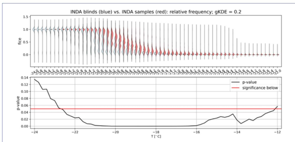
Fig. 4.18.2: Violin plot of ice fraction spectra including all currently analysed samples (red: samples, blue: field blanks). The sampling period ranges from February 2019 until December 2021 with weekly to biweekly resolution.
