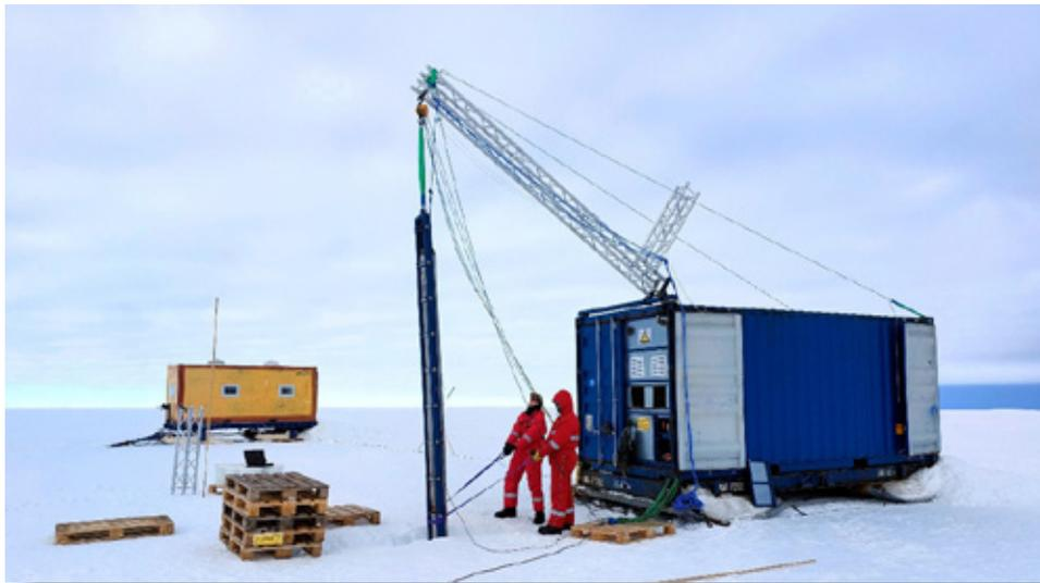
Fig. 4.26.2: Deployment of the TRIPLE-IceCraft Melting Probe
