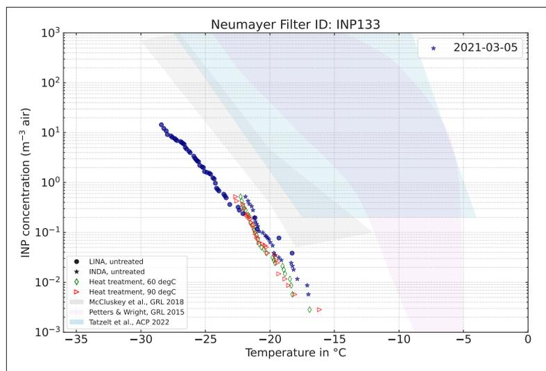
*Fig. 4.18.1: Example of INP freezing spectra (blue area: Tatzelt et al., 2022, grey area: McCluskey et al., 2018); sample period was two weeks, the date gives the start day of the sampling period. Each filter is analysed with two different freezing arrays covering by this a wider freezing range. Besides the samples are heated to  $60^\circ\text{C}$  and  $90^\circ\text{C}$  to gain information on the fraction of heat-labile ice active protein.*
