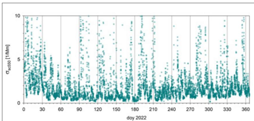
Fig. 4.2.4: Time series of aerosol scattering coefficient at 550 nm,  $s_{sp}(550)$ , measured with an integrating nephelometer (TSI Model 3563). Presented data are one-hour averages based on originally one-minute data.
