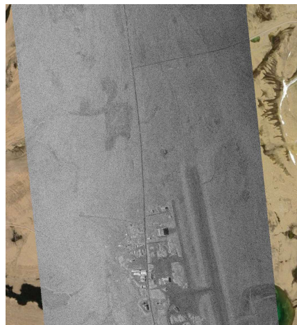
Figure 13: CryoSAR image (Ku-VV) of part of the Resolute airport. The runway and airport were overflown repeatedly on April 27 for calibration of ALS, MACS, and CryoSAR.
