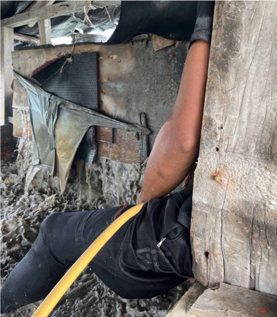
Figure 3. A tin diving member sitting atop seabed sediments mixed with tin ores on a wooden floating raft, holding a yellow breathing pipe.
