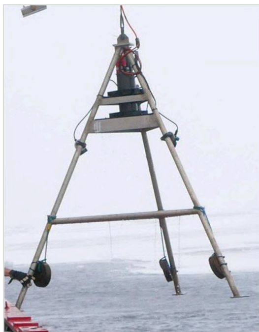
Figure S1. British Antarctic Survey's Shallow Underwater Camera System (SUCS). Photo credit: David Barnes (Bridges et. al, 2021).
