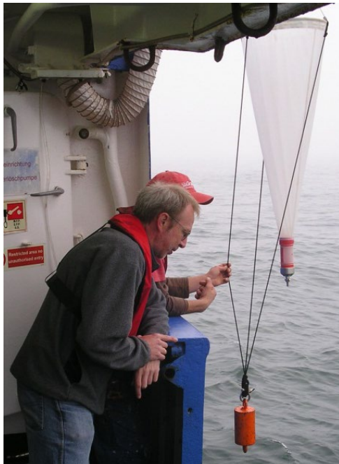
Plankton net Pore size 20 \mu\text{m}
