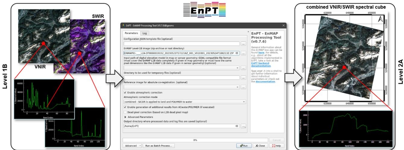
Fig 1: Visualization of the EnMAP pre-processing from Level-1B to Level-2A with the EnMAP Processing Tool (EnPT)
