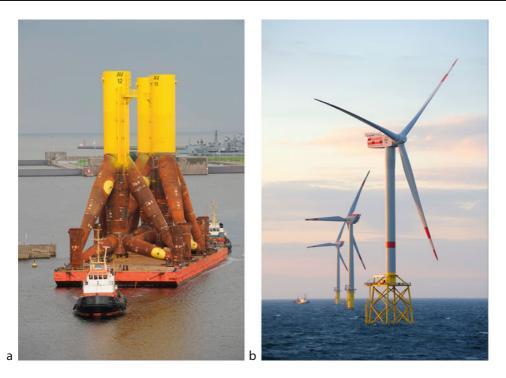
Aquaculture and Renewable Energy Systems, Integration of. Figure 3 Offshore wind farm Alpha Ventus. (a) Shows the transfer of the windmill tripods to the harbor of Wilhelmshaven and (b) displays the setup of an offshore windmill (REpower MI 068 [39])
