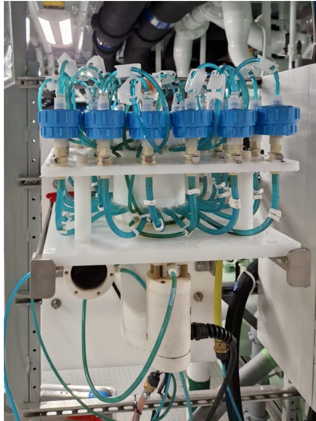
Fig 8.2: The PPS (Particle and Phytoplankton Sampler) installed on board of MS Fridtjof Nansen
