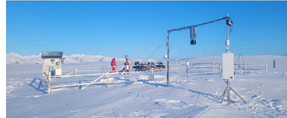
Fig. 4. a) One of the POLA-R muon detectors installed at Ny-Ålesund. The orange dots mark the position of the SiPM devices on opposite corners of the four scintillator plates. b) The Bonner Sphere Spectrometer (BSS) installed at Ny-Ålesund, c) The cosmic-ray neutron sensors (CRNS) installed at the Bayelva site at the outskirts of Ny-Ålesund.
