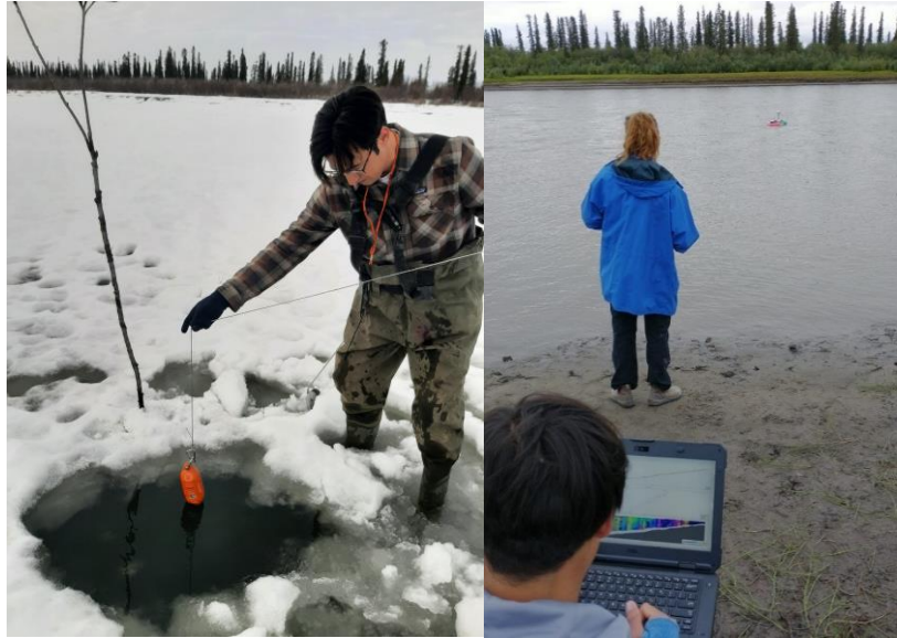
Fig. 2.4: CTD Cast Away measurement during winter (left) and RiverSurveyor discharge measurement during ice-free period (right) in the East Channel in Inuvik
