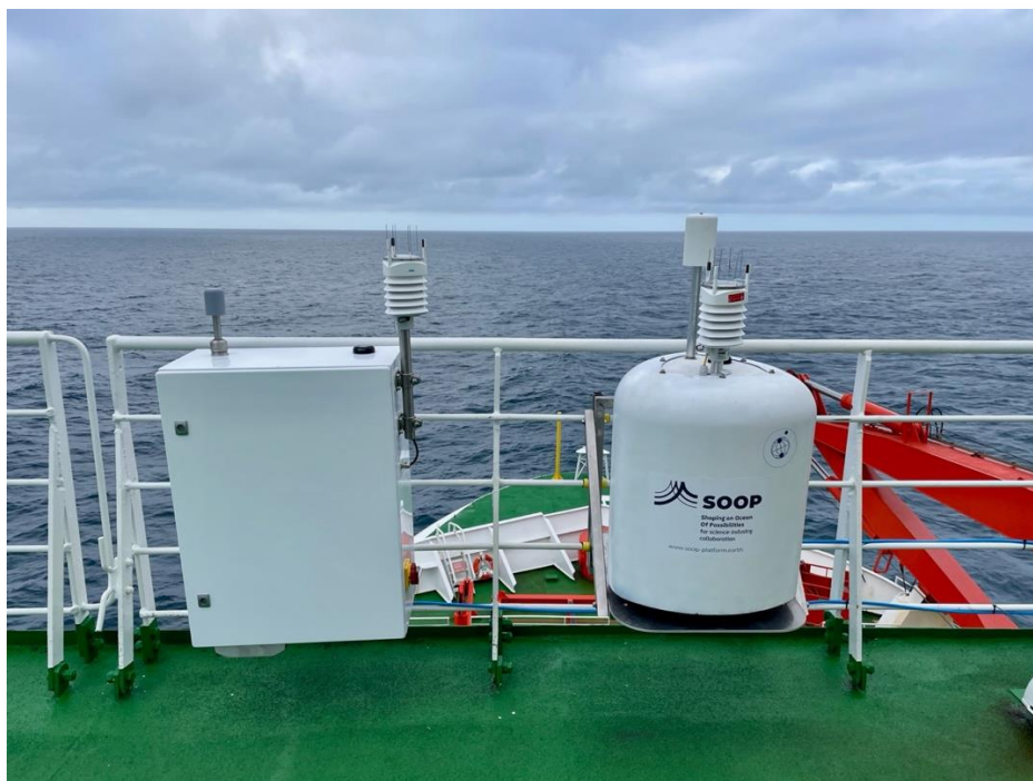
Fig. 2.1: PAMOS 001 (right) and PAMOS 003 (left) installed on the upper observation deck of Polarstern during PS147
