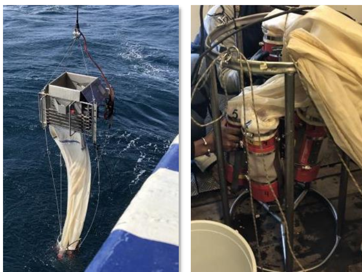
Fig. 5.3: MultiNet sampler used during PS147/2 for the collection of zooplankton samples
