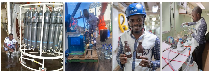
Fig. 5.4: Neuston and planktonic sampling procedure during PS147/2: Sampling process from Niskin bottles (left), incubation (middle left), Lugol samples (middle right) and filtering process (right)
