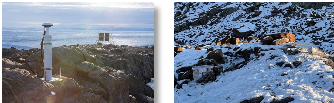
Fig. 5.2.3: GNSS installations at Lambert Land West (LAP1, 2022, left) and Peary Land (PEAR, 2025, right). At LAP1 the GNSS antenna is mounted on top of a special pillar fixed to bedrock. Receiver, batteries and further equipment are stored in two Zarges aluminium boxes (mounted at the structure in the background), while four solar panels and a wind generator are used to recharge the batteries. At PEAR (right) the receiver and batteries are in the Zarges box (left), antenna and solar panels are mounted on bedrock (right).
