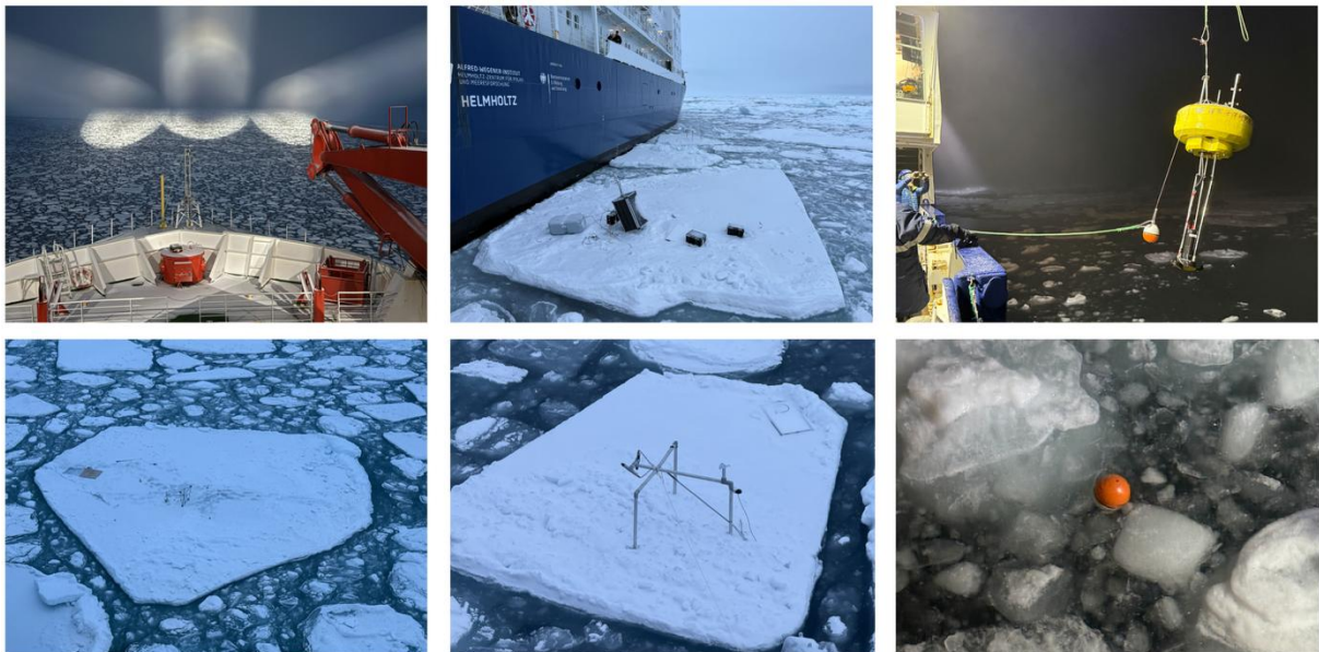
Fig. 4.8.1: Photographs from the buoy recoveries on 8 September 2025. These buoys were deployed on Regime 3 of the CONTRASTS expedition and recovered at the end of their life time (see Figure 4.0.1): A) sea ice conditions in the marginal ice zone during recovery, B) Camera Buoy 2025K3, C) Acoustic Current Doppler Profiler, D) Snow Buoy 2025S133, E) Radiation station 2025R29, F) position buoy from the former meteorological tower. (Photos: Marcel Nicolaus, AWI)
