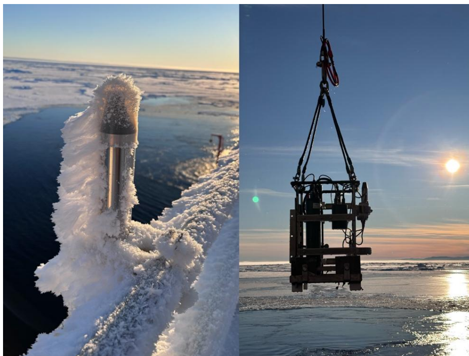
Fig. 3.4: RAMES radiometer sensor mounted above Deck A to measure the sunlight irradiance (left) and the light profiler (right)
