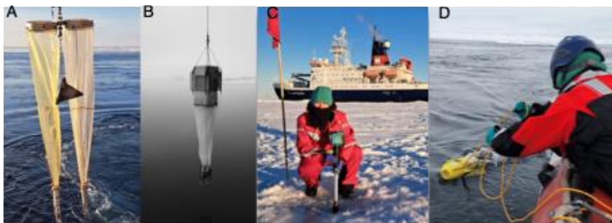
Fig. 3.7: Gear deployed by the ARJEL team on PS150; (A) Bongo net, (B) Multi-net, (C) PK 1 pump sampler, (D) Yellow submarine sampler. Photo credit: Rebecca Gorniak
