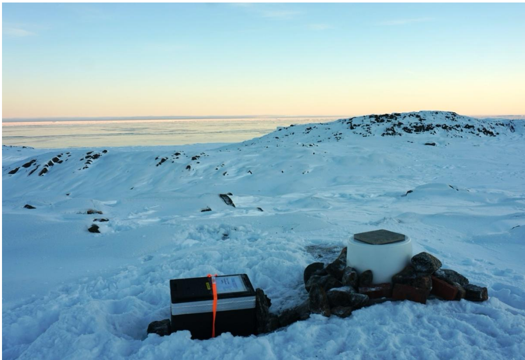
Fig. 5.1.4: Fully mounted seismic station on land. The seismometer is covered by the bucket, data recorder and battery supply are contained in the insulation box.
