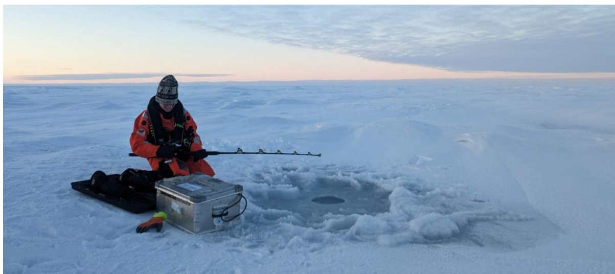
Fig. 2.29: An RBRconcerto CTD is deployed through an ice hole during a helicopter-based station using a motorized fishing rod. The Zarges box contains the mobile Simrad Echosounder to determine the water depth beforehand. Photo by Manuel Franco Pire.
