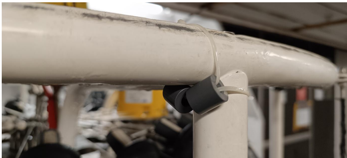
Fig. 2.7: POM parts provided by the BSH for their ArgoFloats attached to the CTD. Photo by Mario Hoppmann.
