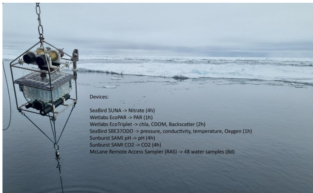
Fig. 7.2.1: Biogeochemical sensor package: SeaBird Suna (NO 3 ), Wetlabs Ecopar (PAR), Wetlabs EcoTriplet (CDOM, chl a , backscatter), SeaBird SBE37ODO (CTD + O 2 ), Sunburst Sami pH (pH), Sunburst Sami CO 2 (CO 2 ), McLane remote access sampler (48 water samples)
