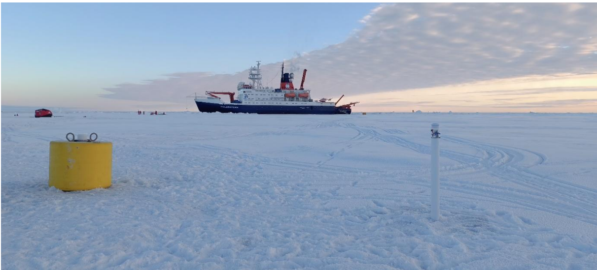
Fig. 2.34: Photo of ice-tethered profiling buoy TOP016 (2025W17, left) and seasonal ice mass balance buoy 2025F (2025I18, right) during ice station 3 on 25 September 2025. Photo by Mario Hoppmann.
