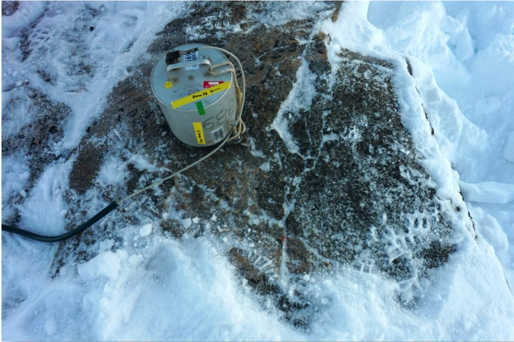
Fig. 5.1.3: Seismometer installed on bedrock
