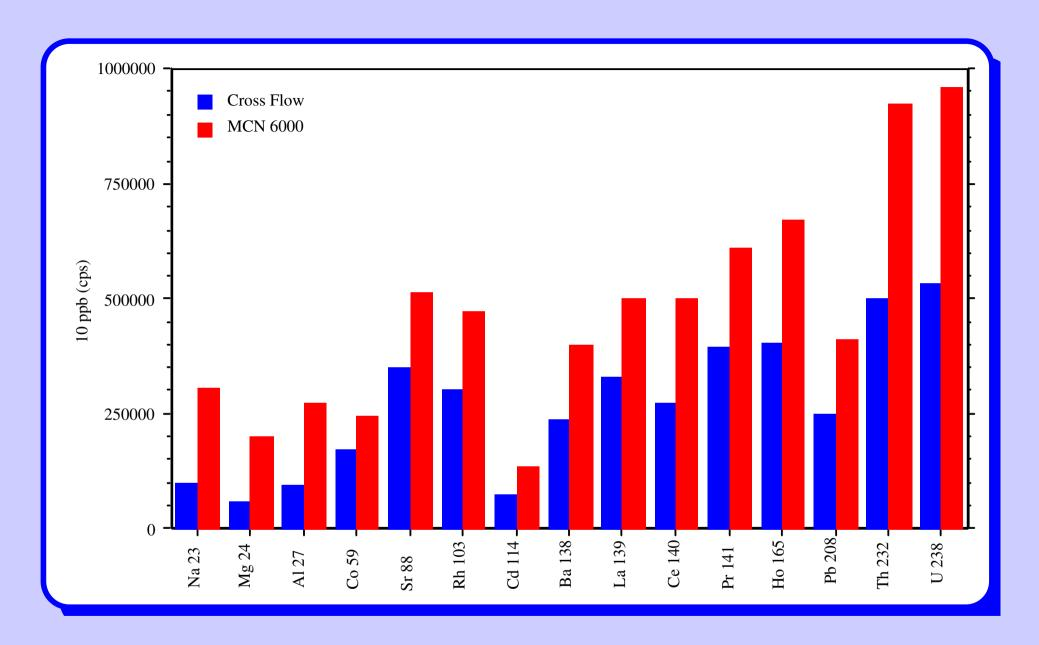
Intensities (cps) for a 10 ppb multielement solution by using a Cross Flow Nebulizer and a microconcentric Nebulizer with membrane desolvatisation kit (MCN 6000)
