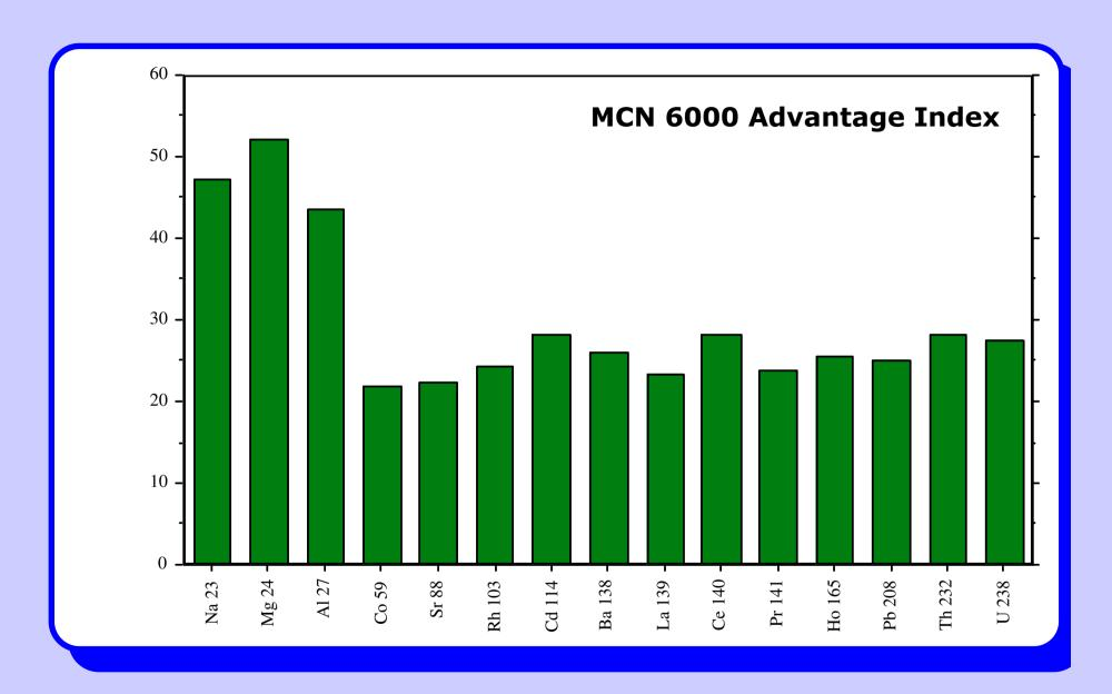
Advantage index for a MCN 6000 in comparison to a Cross Flow Nebulizer for a 10 ppb multielement solution, defined as relative Sensitivity/Sample uptake rate (Cross Flow Nebulizer = 1)
