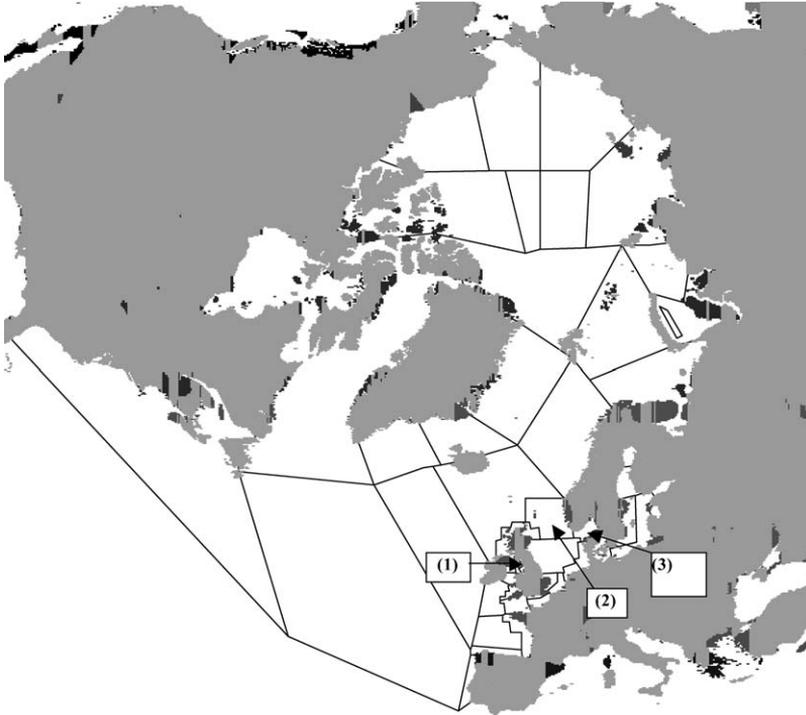
Fig. 6. The structure of the surface water boxes of the NRPA box model with three boxes used for the intercomparison in Fig. 4 (1—Cumbrian Waters; 2—the northern North Sea; 3—Skagerrak).
