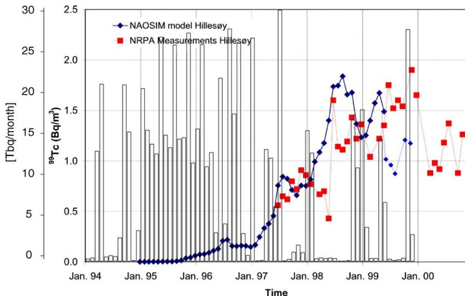
Fig. 1. Time series of the release function at Sellafield (bars), and surface concentrations from observations (squares) and NAOSIM results (rhombs) near Hillesøy at the northern Norwegian coast near  $69^{\circ}\text{N}$  for the period 1994–1999.
