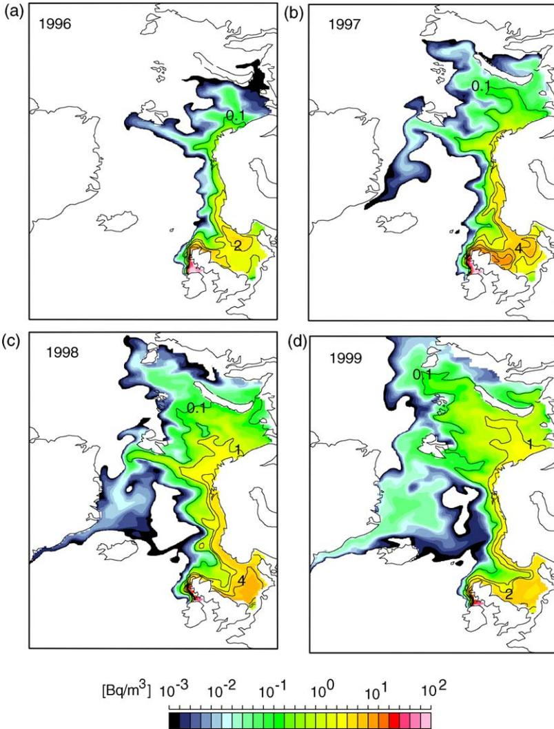
Fig. 2. Distribution of <sup>99</sup>Tc (Bq/m<sup>3</sup>) in surface water in September (a) 1996, (b) 1997, (c) 1998 and (d) 1999, from model results (lines 0.1, 1.0, 2.0 and every 2.0 Bq/m<sup>3</sup>).
