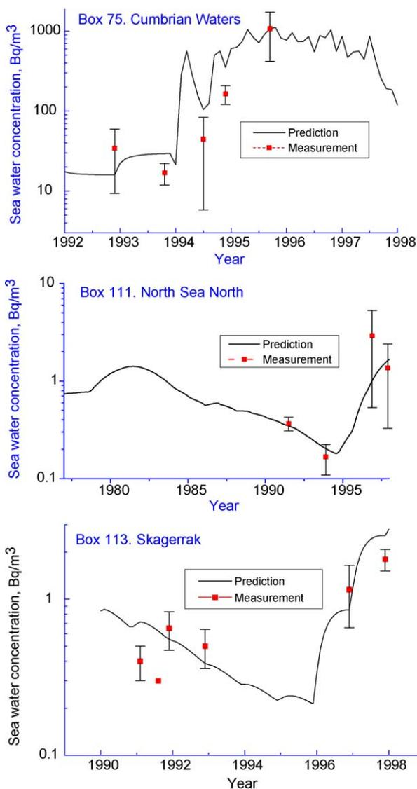
Fig. 4. Comparison of box model concentrations of  $^{99}\text{Tc}$  for individual boxes and experimental data. The solid lines correspond to the results of calculations executed by the NRPA box model. Squares show the average values for the marine compartment with one standard deviation for experimental data.
