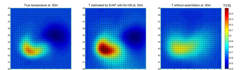
Temperature  $T$  at 50m depth at the end of the assimilation period. Shown are (from left to right) the true temperature field, that estimated by the EnKF filter with  $N=100$ , and  $T$  from a simulation initialized as the filters, but without assimilation.
