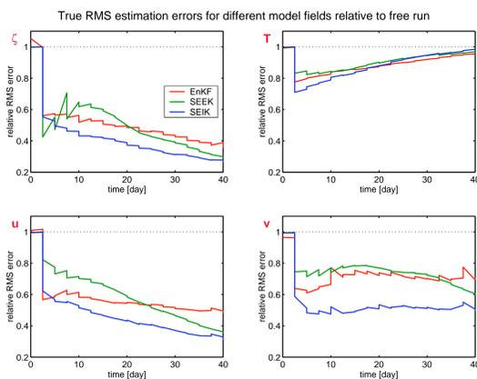
RMS estimation errors for the four model fields for assimilation with an ensemble size of  $N = 10$ . The RMS values are scaled by the RMS deviation of a simulation without assimilation from the true state fields.
