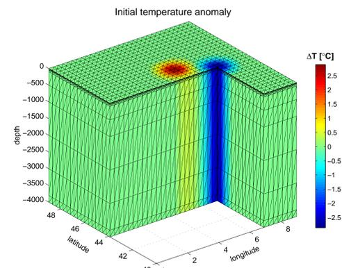
Cut into the model domain showing the initial temperature anomalies and the tetrahedral finite element discretization.
