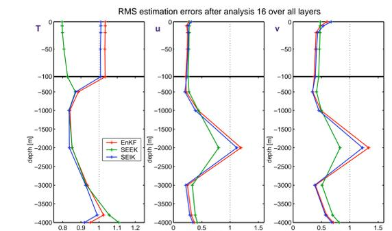
Relative RMS estimation errors at the end of the assimilation period displayed over all layers for  $N = 100$ .
