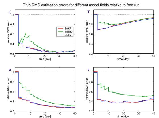
RMS estimation errors for the four model fields for assimilation with an ensemble size of  $N = 100$ . The RMS values are scaled by the RMS deviation of a simulation without assimilation from the true state fields.
