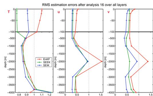
Relative RMS estimation errors at the end of the assimilation period displayed over all layers for  $N = 10$ .
