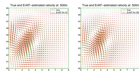
Comparison of true and estimated velocity fields at 500m depth at the end of the assimilation period. Shown are the true velocity field and the velocity estimated using the EnKF with  $N=10$  (left) and  $N=100$  (right).
