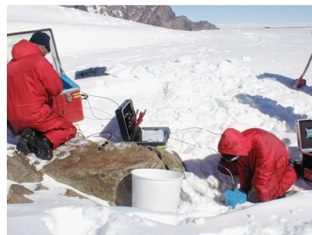
seismometer set up at Weigel Nunatak (KOTA) Kottas Mountains, Antarctica
